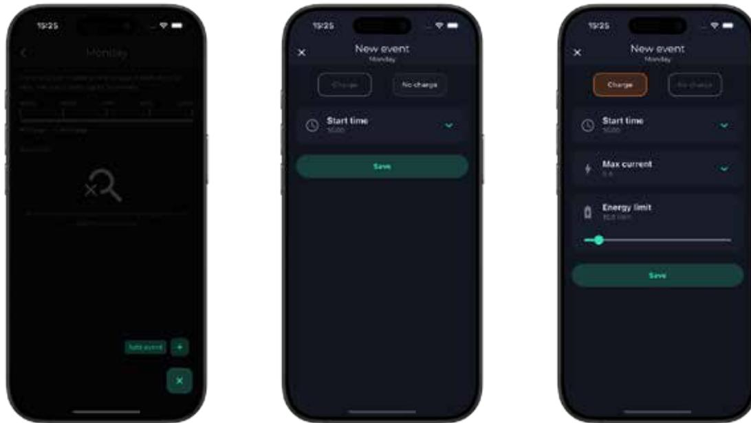
Click on the „add event“ button. Choose the time to start charging, the charging current, and the limit of kWh you want to charge. (If the value is 0 kWh, charging will stop only at the limit set in your electric car or at the selected charging end time.) Select whether you want to start or stop charging during this event.
